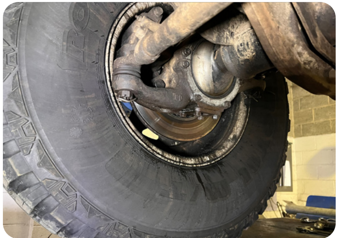
Oil leak from brake hub and oversize tyre fitted
