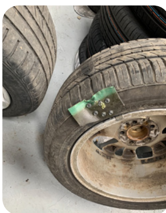
Hand patched tyre side wall
