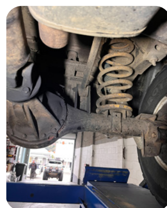
Anti roll bar removed
